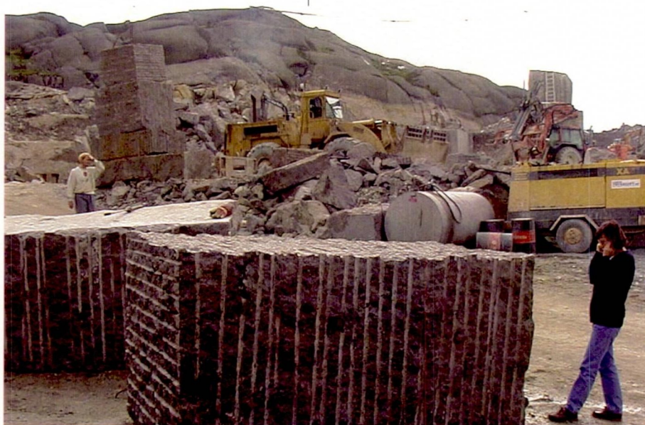
A popular, new type of block is labradorite antique, an anorthosite from Oгна, Hå, Rogaland, produced by Granitt 1893 A/S and NSSI A/S.
