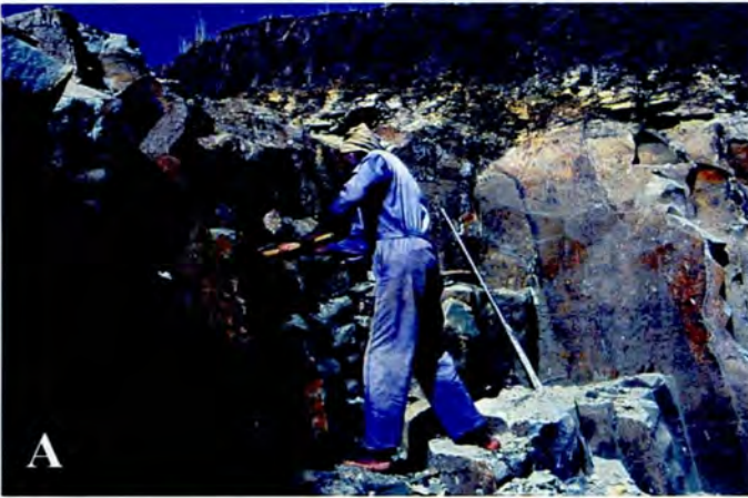
Figure 33 Ignimbrite in Addis Ababa. A) Quarrying with sledge and wedges. B) Ignimbrite in the Catholic Church, Addis Ababa. C) Ignimbrite in the Cathedral, Addis Ababa.
