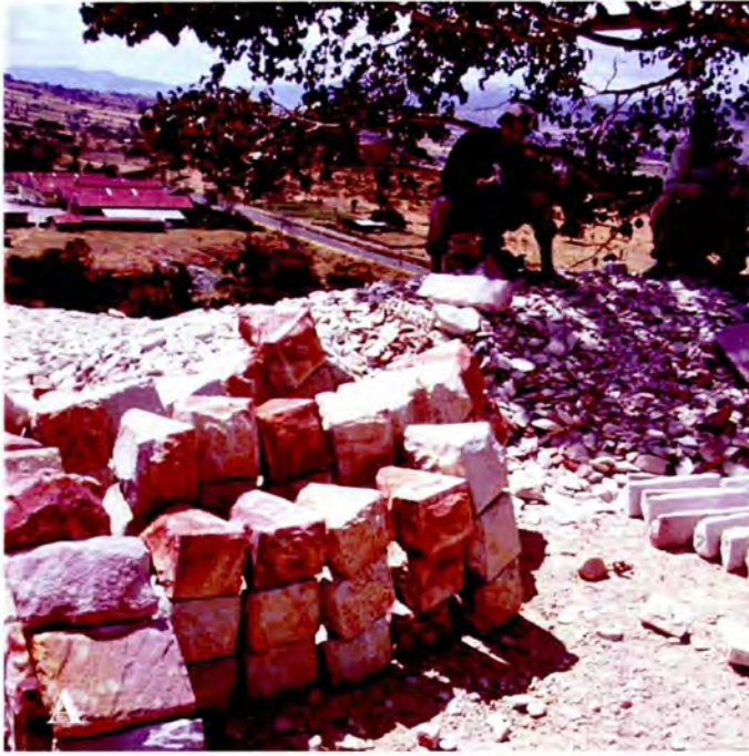
Figure 31 The Ambo sandstone. A) Shaping sandstone blocks. B) Quarry. C) Sandstone wall in Addis Ababa.
