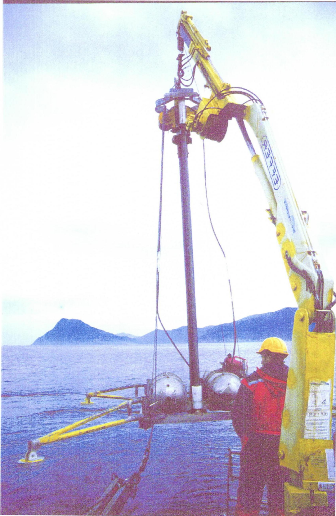
Fig. 3. The vibracorer HYBAV operated from FF "Seisma" (Photo: John Howe)
