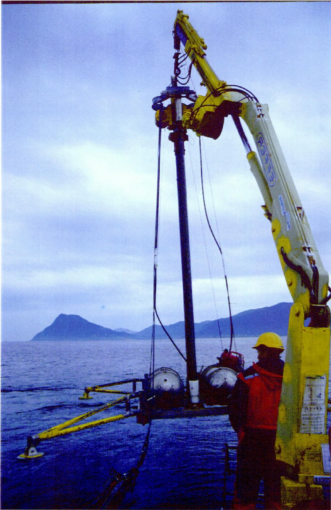
Fig. 11. The vibrocorer HYBAV operated from RV Seisma.
