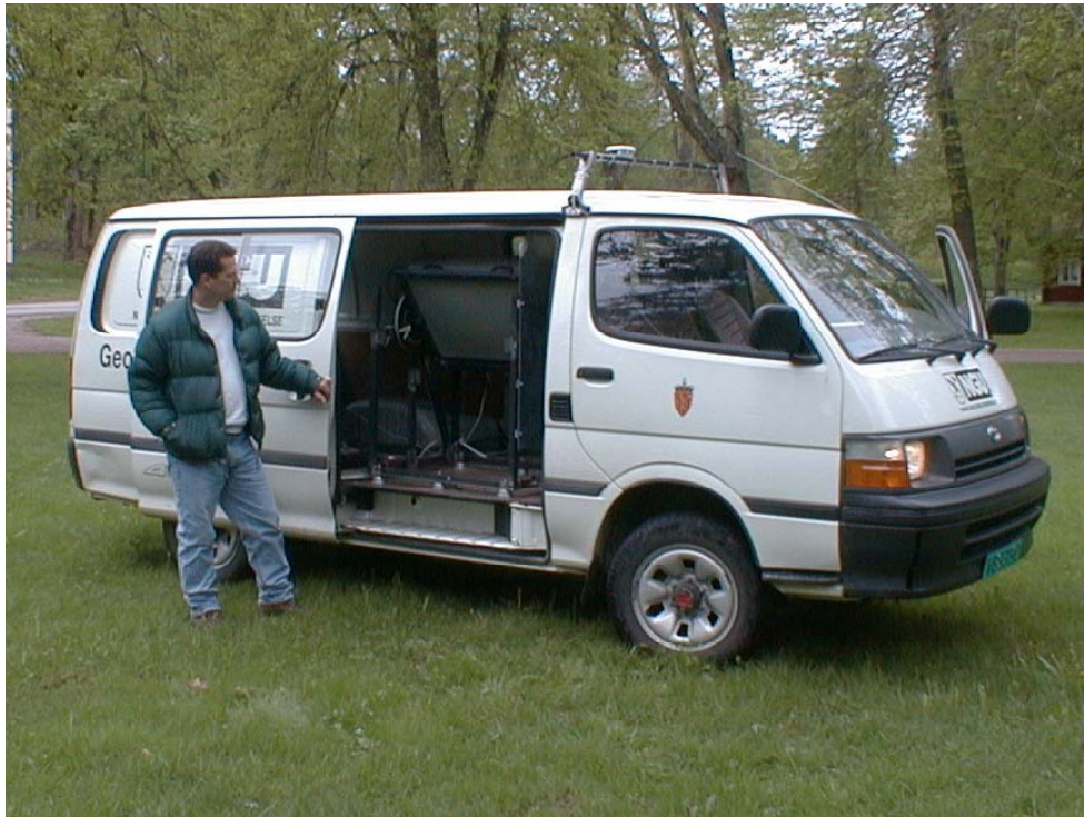
Figure 2. The measuring system used by team NOK of the Geological Survey of Norway. Note that the 16.7 litre NaI detector behind the side door can be rotated to present a larger cross-sectional area to the left and right sides of the road.
