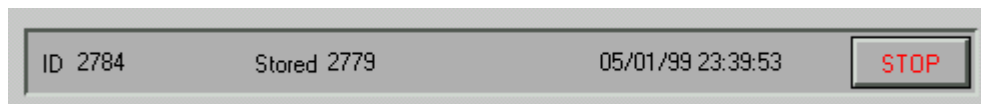
Figure 11. Logging status. From left to right: 'ID' - logging cycle number used as data record number in data files; 'Stored' - number of records written to data files; date and time from spectrometer; program 'stop' button (terminate logging).
