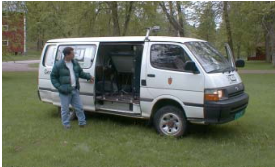
Figure 1. The Geological Survey of Norway's car-borne gamma ray spectrometer system. The NaI gamma ray detector is visible through the side door.
