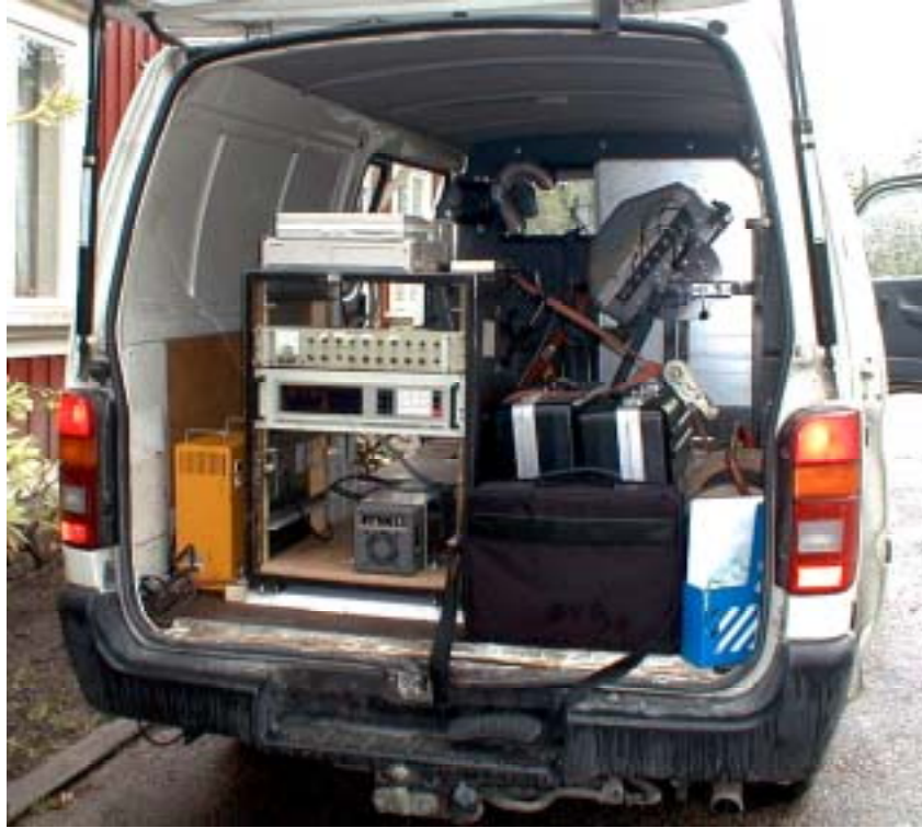
Figure 3. The instrument rack mounted at the rear of the car. The NaI detector is visible in the background next to the side door.
