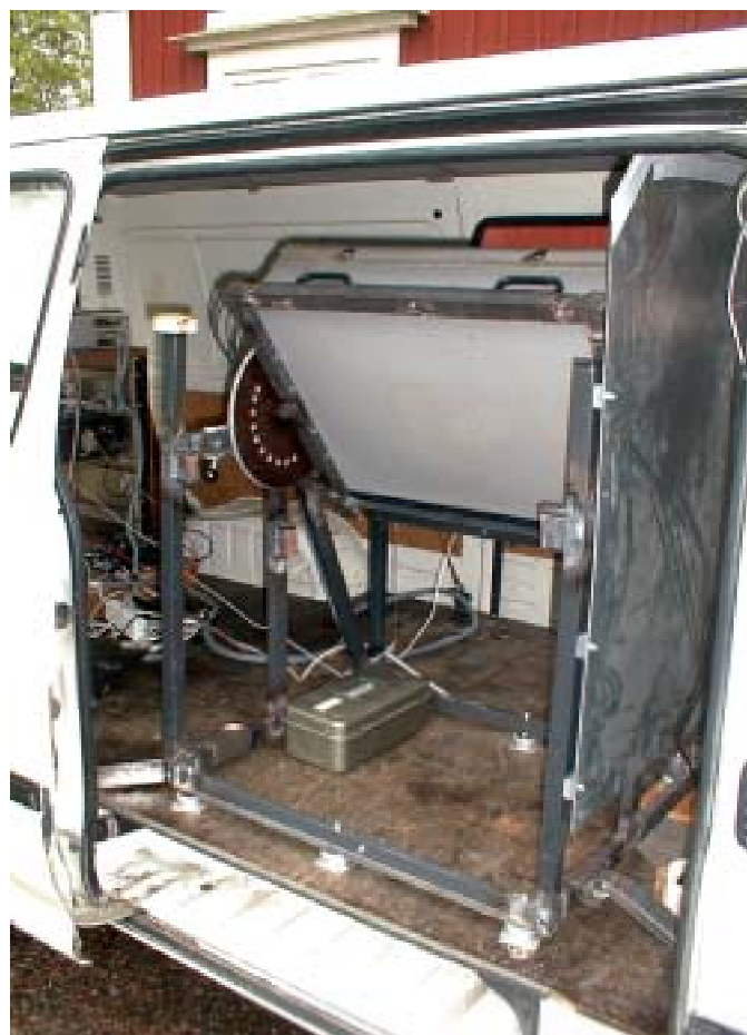
Figure 2. A close-up view of the NaI detector and the frame that supports it. The tilt angle of the detector can be adjusted so that it registers more gamma rays from the roadside than from the road itself.
