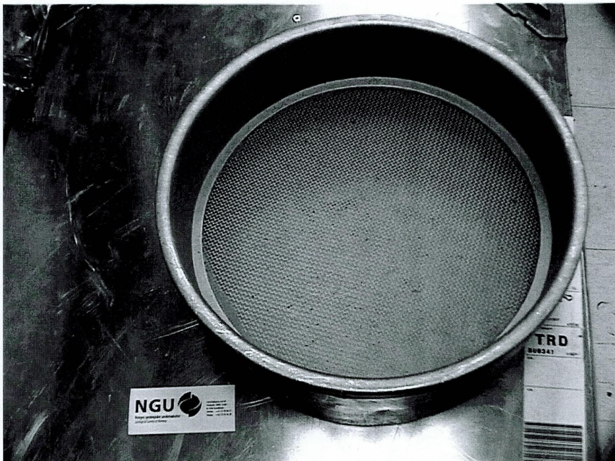
Figure 1. Sieve used in the field for sieving stream sediments.
