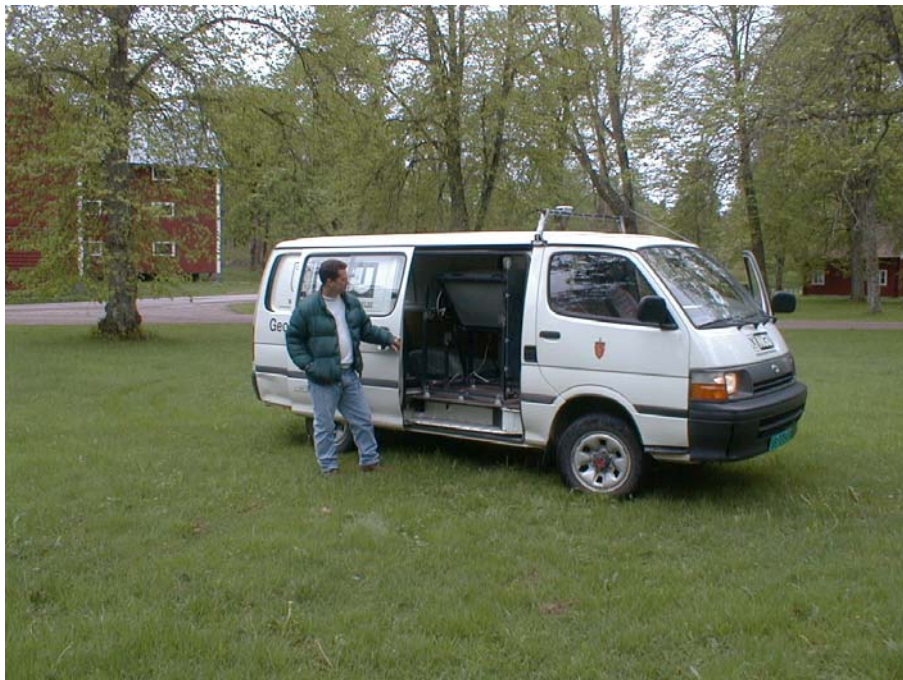
Figure 3. The NGU's vehicle and measuring system at the calibration site at Älvkarelö Herregård. This photo was taken in May 2000 when NGU measured the RESUME-99 fixed route. The side door is open so that the large NaI detector can be seen tilted towards the right side of the vehicle. The door is closed under normal operation of the measuring system.
