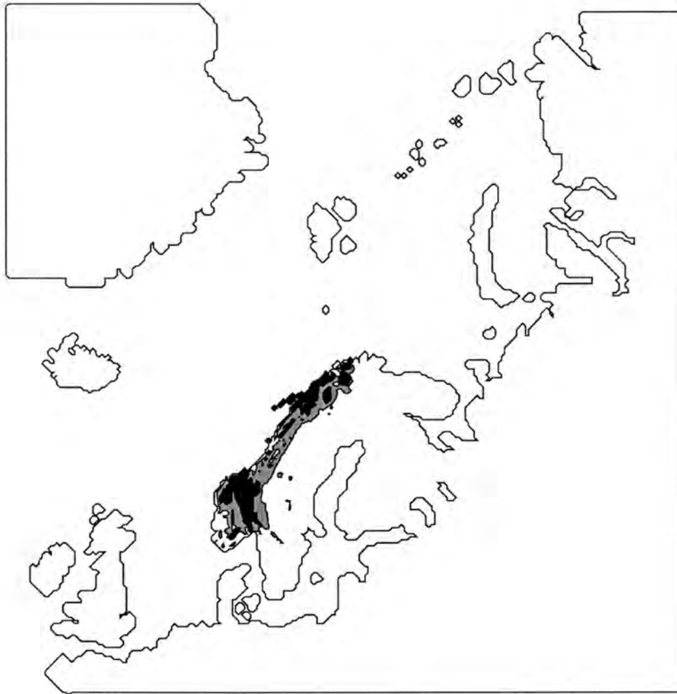
Fig. 7.1.10 Areas with significant positive deviations (>1,0 mm/yr) between the observations and the calculated glacial isostatic uplift.
