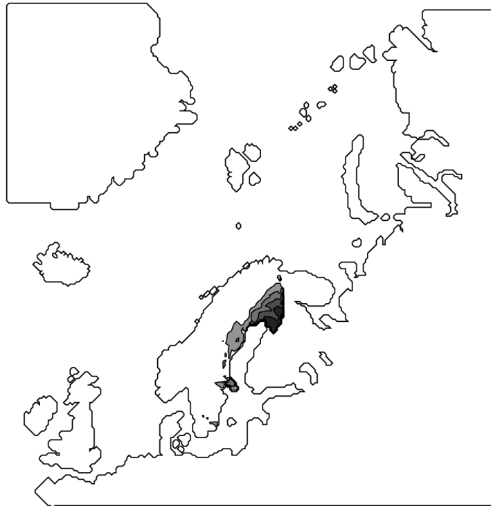
Fig. 3.2.6 Areas with significant negative deviations (grey areas >0.5\text{mm/yr} ; black areas >1.5\text{mm/yr} ) between the observations and the calculated glacial isostatic uplift.
