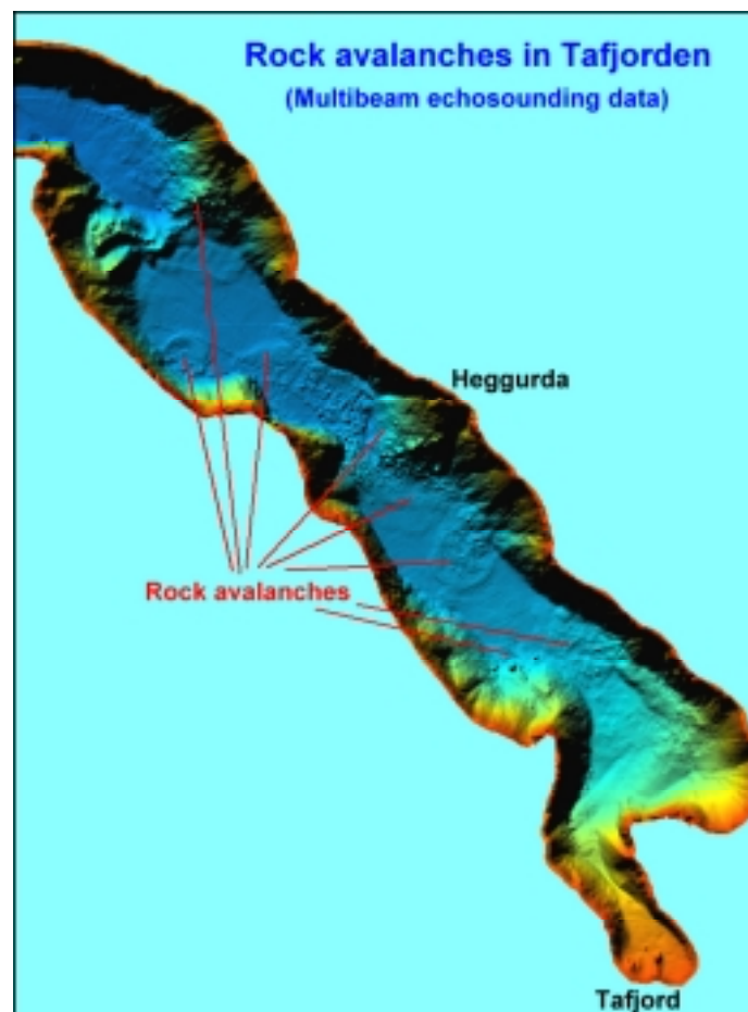
Fig. 1.4.7 Large rock avalanches in Tafjorden, Møre & Romsdal. The shaded-relief map covers ca. 8 km of the fjord.
