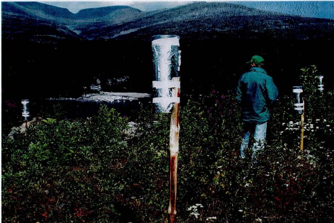
Fig. 2. A typical precipitation sampling station as used during the Kola Project. Note that the Kola sampler had different dimensions than the one used for the Barents Project. The station is set up in an open place so that no throughfall from trees or bushes can influence the results.
