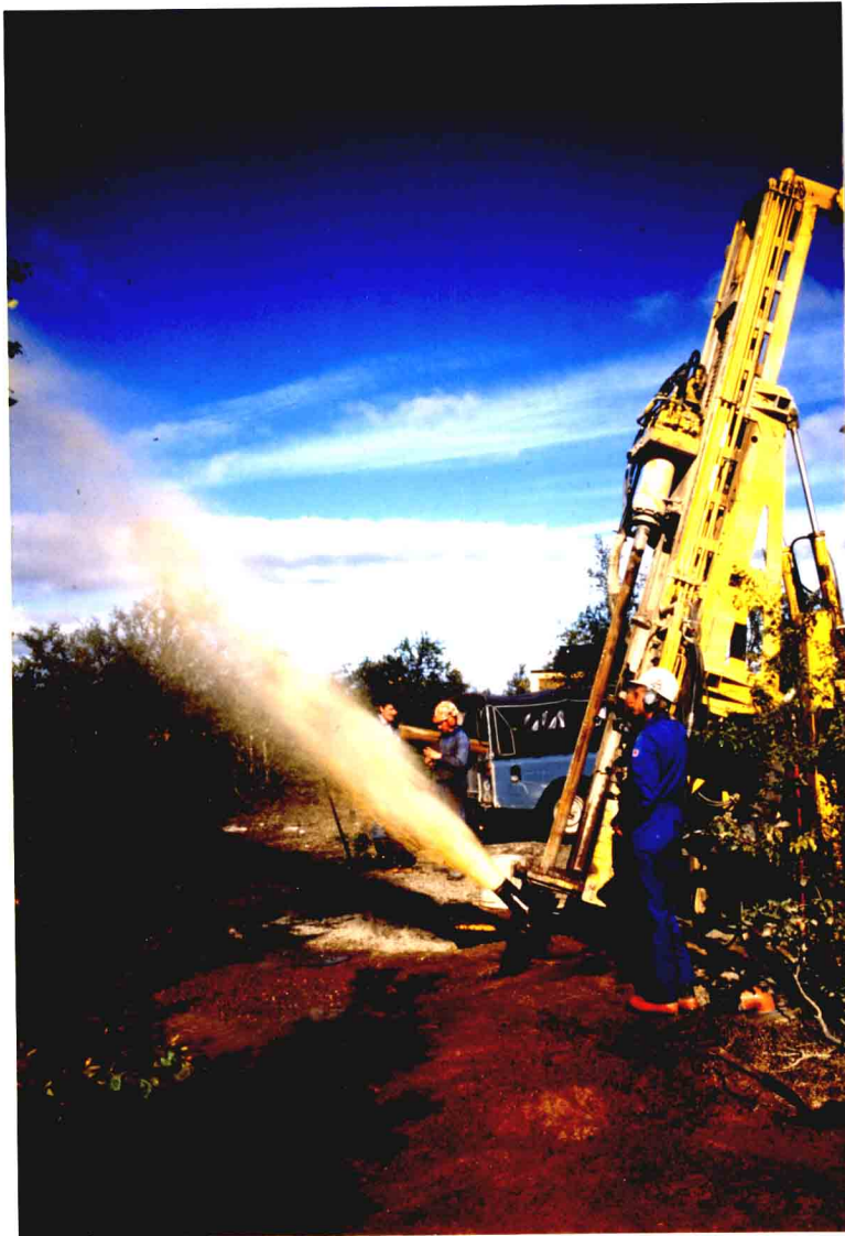
Figure 6. Percussion drilling through the Stuoragurra Fault in the Skarrejavri-Fidnajaikka area showed high content of groundwater in the fault zone. The yield was estimated to minimum 17 m 3 /hour (Klemetsrud & Hilmo 1999) which was the capacity of the most powerful pump available for a 5.5" diameter well. This borehole yield is among the highest ever measured in hard rock aquifers in Norway. The well on the picture is emptied by blowing pressured air into it.
