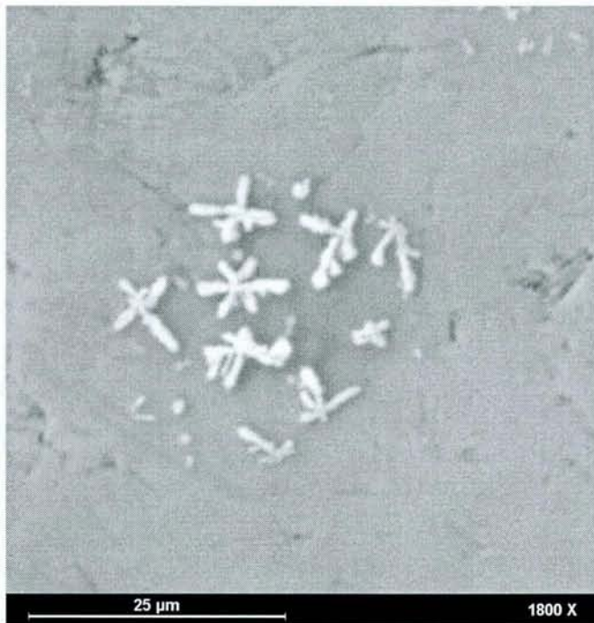
Figure 12: Crystals of sylvine (light-coloured) formed by evaporation. Egyptian talc. Backscattered electron image.
