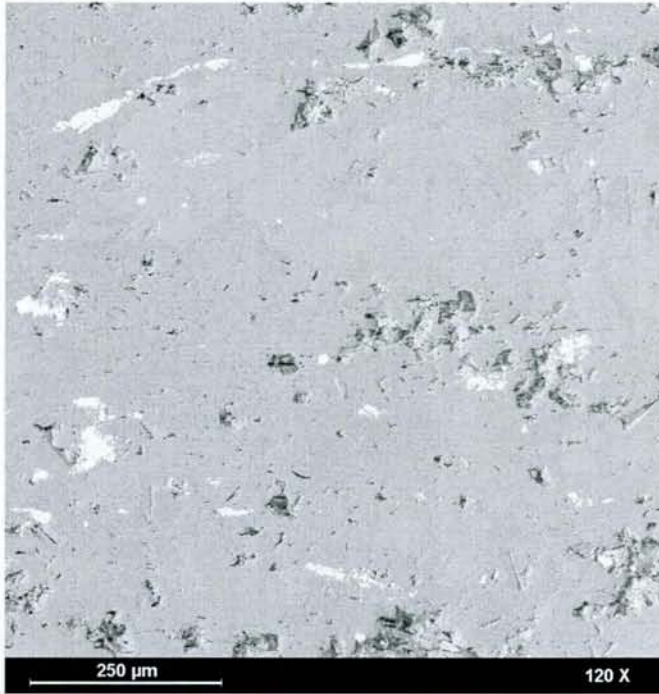
Figure 13 : Sphene (light-coloured ) situated in talc, amphibole and quartz in the Korean talc rock. Backscattered electron image.
