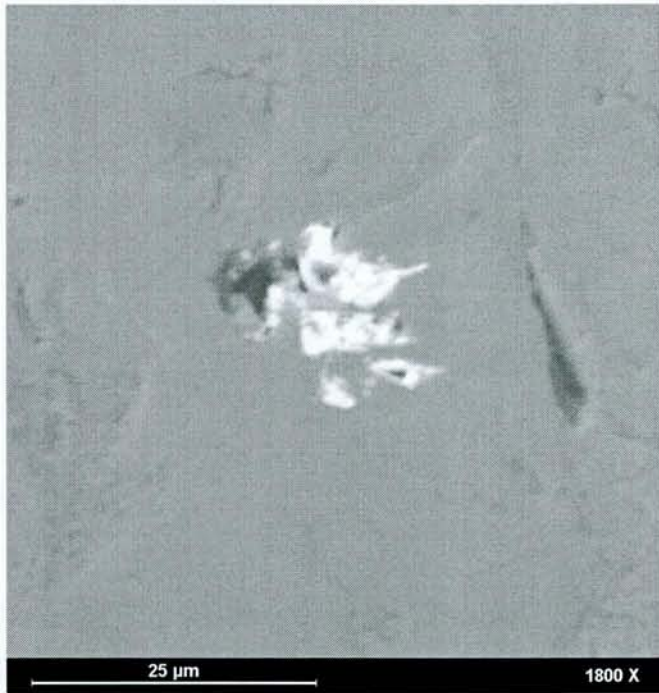
Figure 11: Desert rose of gypsum/anhydrite made by evaporation. Egyptian talc. Backscattered electron image.
