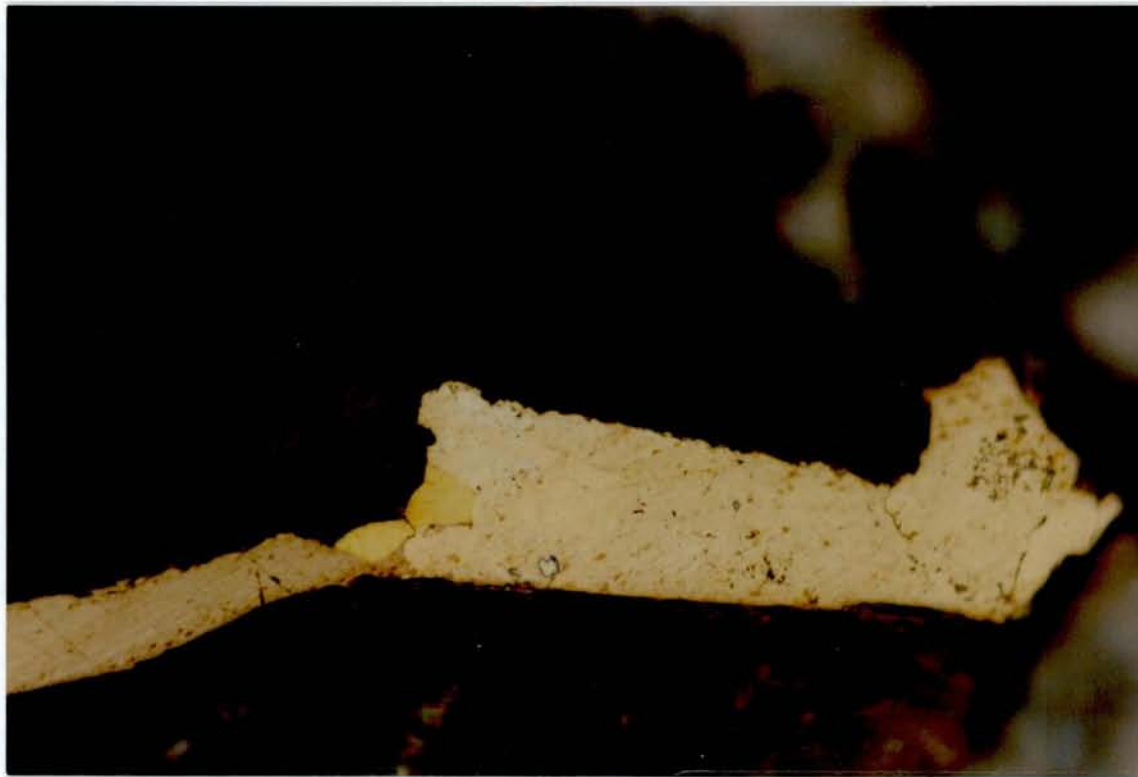
Figure 5 : Microphoto of a sulfide grain carrying three different phases. Altermark talc. Yellow grains in the middle: chalcopyrite, brownish grain to the left: pyrrhotite. Large yellow-brownish grain to the right: pentlandite. II-nicols.
