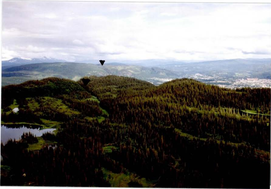
Fig. 2.1.20. Oblique aerial photograph of the Båsmoen Fault (Olesen et al. 1994) on Båsmoffellet, looking east, approximately 4 km to the west of the centre of Mo i Rana in the background of the picture. The fault, shown by the arrows, is trending ENE-WSW and cuts the strike of the bedding (c. NE-SW) at an angle of approximately 20°. The southern block seems to be uplifted. The Båsmoen Mine is located along the continuation of the fault immediately behind Båsmoffellet, in the central part of the picture. The continuation of the BF across Loftfjellet to the east of Båsmoen can be seen in the background.
