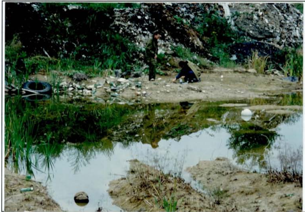
Photograph 7: Sampling soil at the toe of the landfill. This sample, LT54S, containing very high levels of petroleum products.
