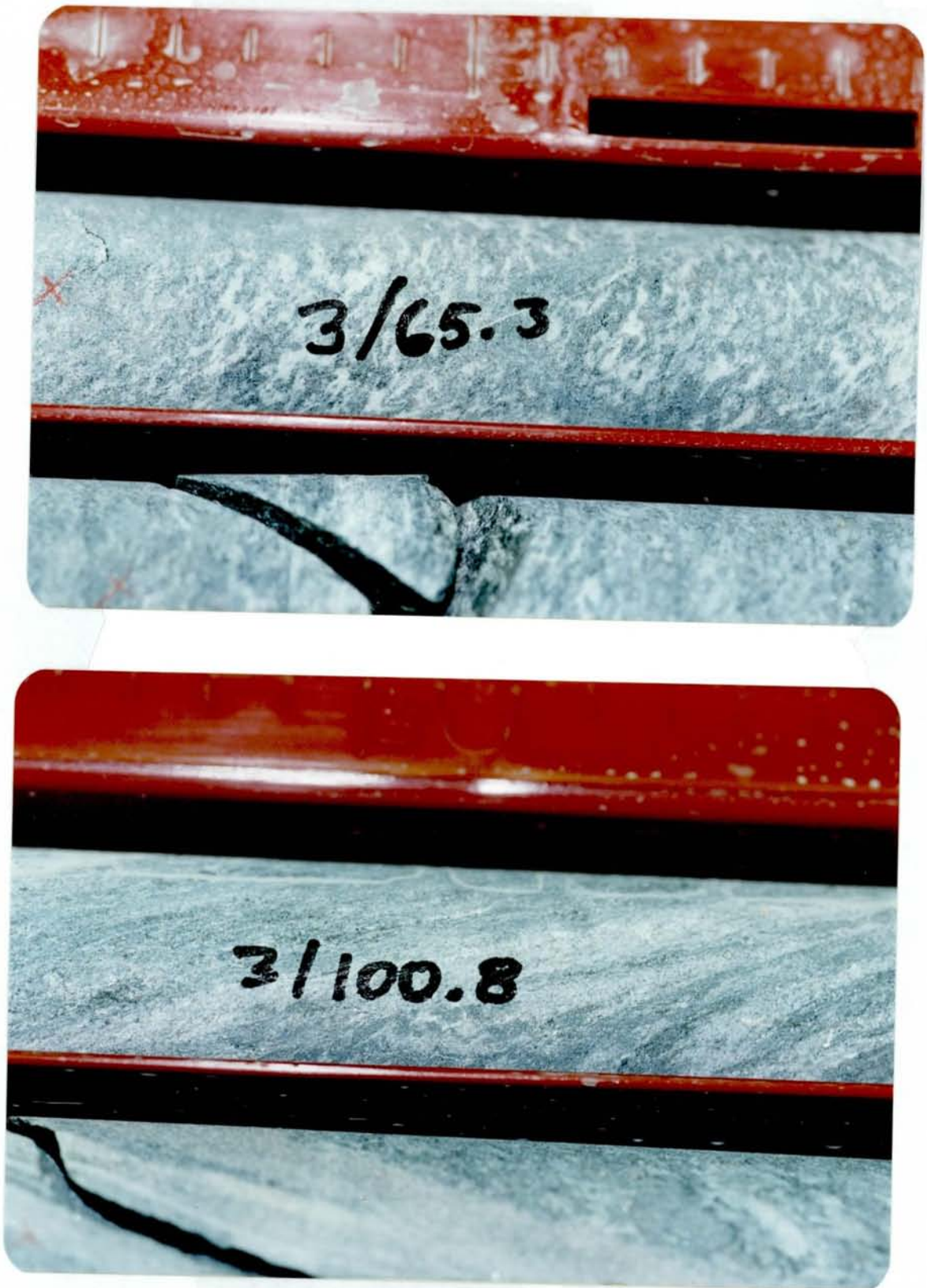
Fig. 7: Upper photo: Eclogite from Dh3 at 65.5 m with preserved gabbroic textures. The white patches are the alteration products after plagioclase, consisting of very fine-grained albite, quartz, white mica and probably also zoisite. The dark patches consist of barroizitic amphibole, omphacitic clinopyroxene and garnet. Lower photo: Deformed variety of the same eclogite as in the previous photograph, but without the preserved gabbroic textures.
