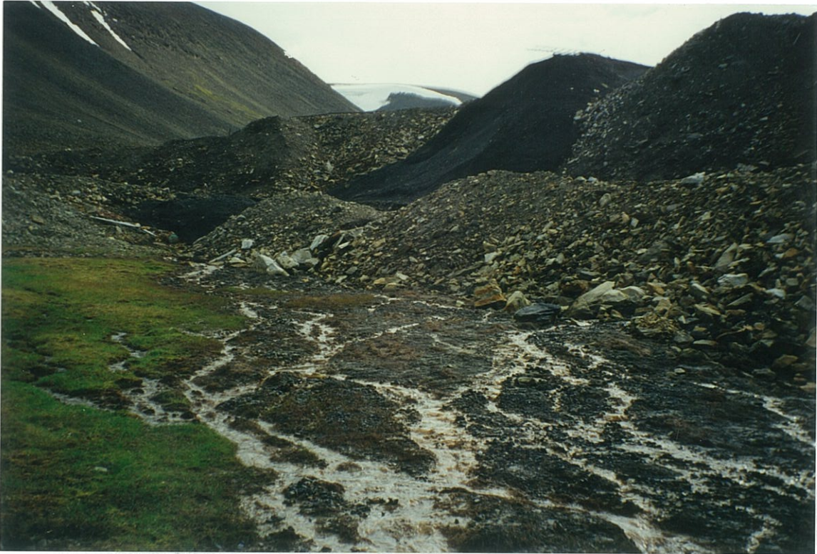
Figure 3c. Leachate from the spoil tip at Mine 3 in Bjørndalen. The sample point was at the head of the seep on the left of the picture.
