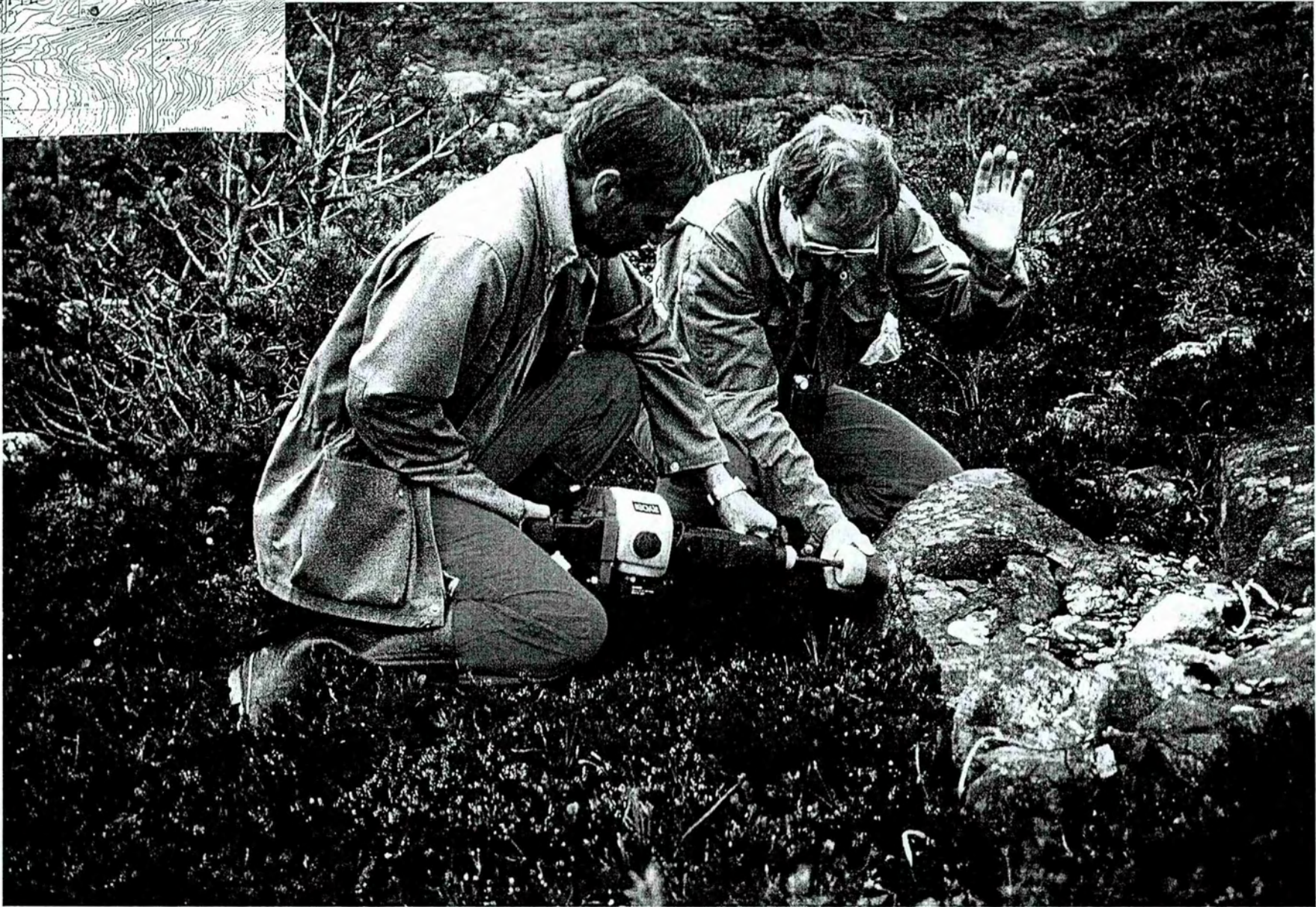
Photograph no. 28: Drill-dust sampling at Orkheia.
