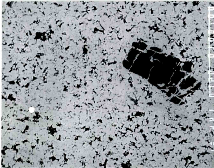
Fig. 16 SEM BEI of carbonated cemented mudstone (?former ash) from core 6814/04-U-02, 36.75 m. The carbonate (light grey, main mineral) is sideritic to ankeritic in composition. The very small light grain is pyrite, whereas the dark grain is a partly dissolved, detrital plagioclase grain.
