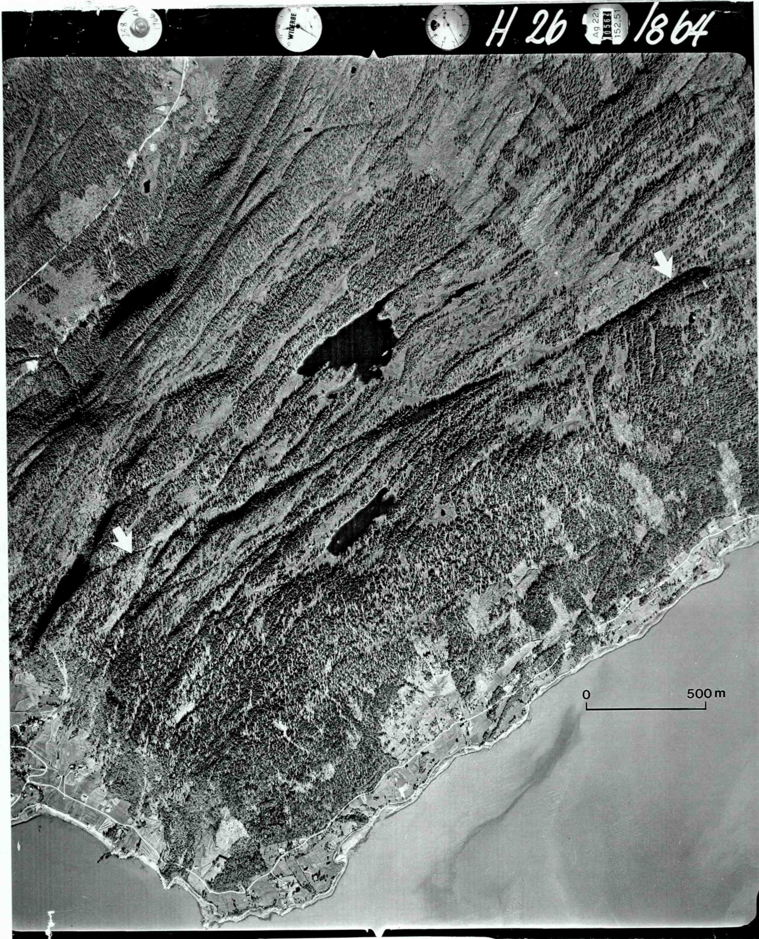
Fig. 13. Aerial photograph of the Båsmoen Fault on Båsmofjellet. The fault, shown by the arrows, is trending ENE-WSW and cuts the strike of the bedding (c. NE-SW) at an angle of approximately 20^\circ . The southern block seems to be uplifted. The Båsmoen Mine is located along the continuation of the fault immediately to the east of the picture. A number of small lineaments parallel to the Båsmoen Fault trend can also be seen on the photograph.
