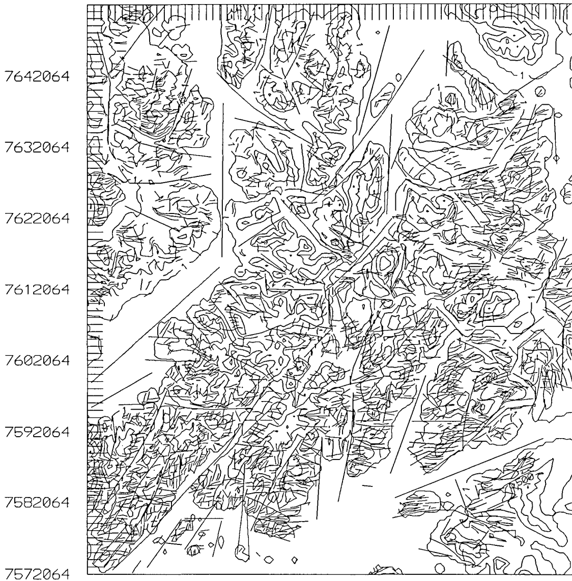
Fig. 7 Result of the lineament interpretation on the island of Hinnøya. This figure shows the interpreted lineaments draped over a topographic map with an equidistance of 250 m. The numbers to the left and above the map are the co-ordinates in the UTM grid 33 W. Tic lines every km.
