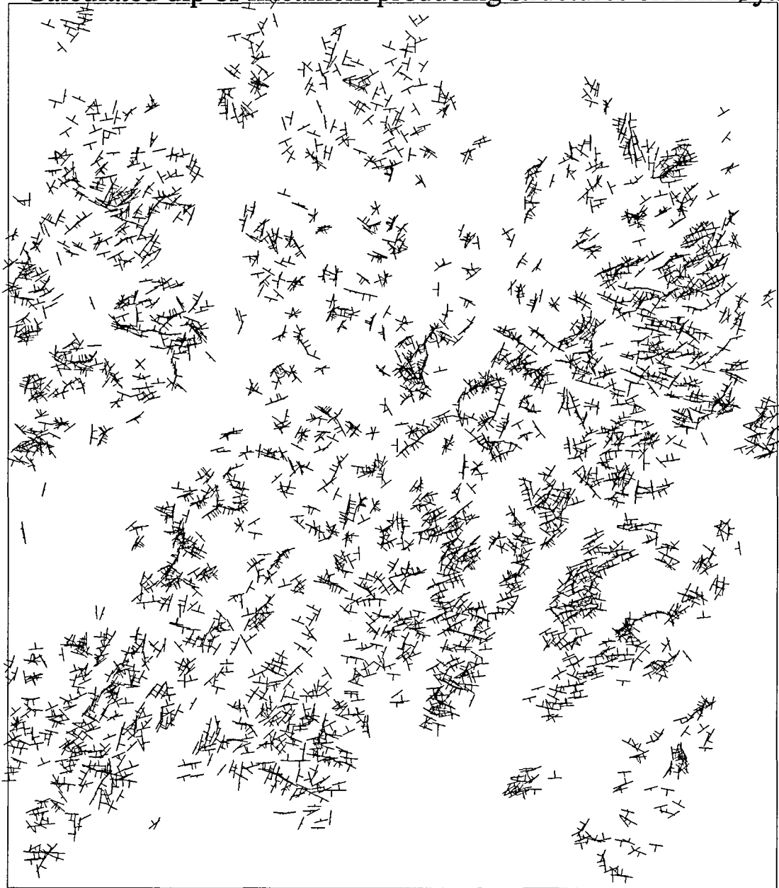
Fig. 9. Calculated dip of lineament segments that were interpreted from Landsat imagery. The elevations at the nodes were used to calculate the dip of every single segment. Compare with the location of the lineaments in the previous figure.
