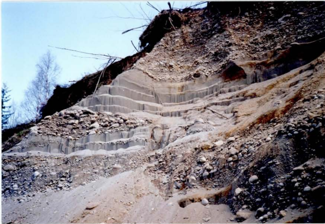
Fig.2(a) Photo of coarse layer at Trandum landfill showing fine and coarse intercalated layers
