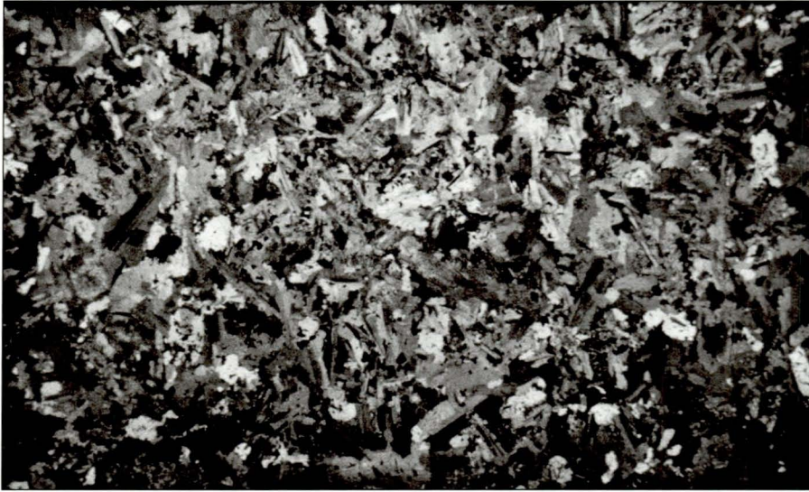
Fig. 5. Photo of whole thin-section of gabbro. Sample no. 72286, crossed polars. The length of the thin-section is 3 cm.
