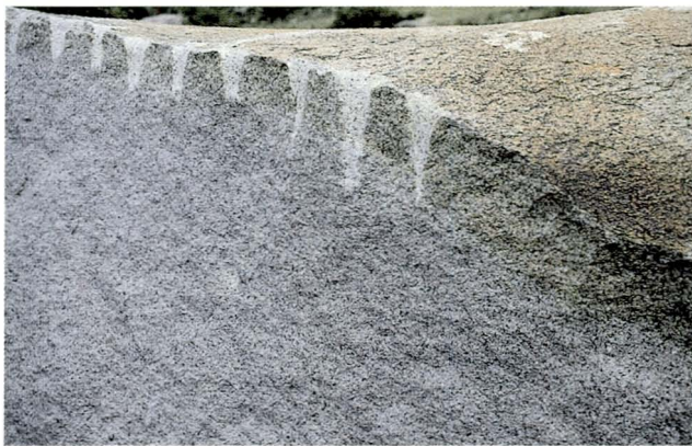
Fig. 5. Split surface of boulder of fine- to medium-grained granite close to Dekemhare. Note wedging holes made by hammer and chisel and stained weathering profile (approximately 7-8 cm in thickness).
