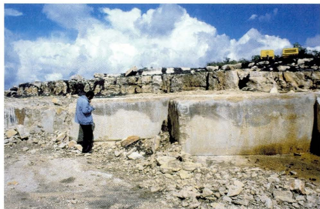
Fig. 9. Sawed limestone bed in a quarry within the Hakimgara limestone deposit, Harar. Note reduction fields in the upper part of the bed.
