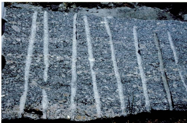
Fig. 8. Raw block surface of the Anger Guten granite in the quarry (cut perpendicular to the foliation). Drillholes are approximately 25 mm wide.
