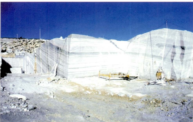
Fig. 3. Diamond wire sawing applied in the Løvgavlen marble quarry, Fauske (northern Norway).
