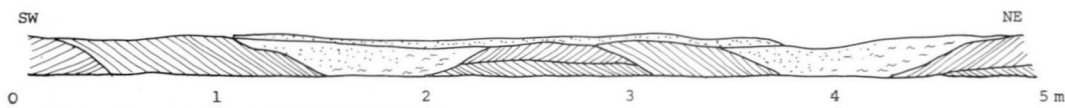
Fig. 48. Series of facies A cross sets showing current reversal and bedform modification in a bed about 13 m above the base of member D at Stappugieddi north. Currents flowed NE, SW, NE, and following a final phase of erosion the troughs were filled with massive and flaser-bedded very fine sandstone.
