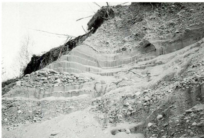
Fig. 4. Sediment texture at the Trandum landfill, in the side-wall of the kettle hole. Note the abrupt changes in grain-size which strongly influence the hydraulic parameters.
