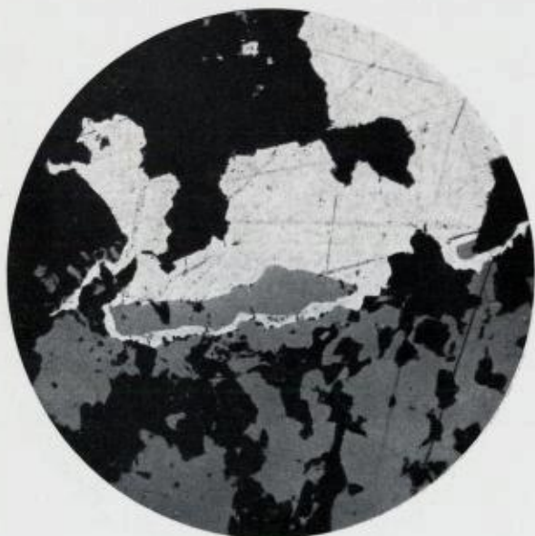
Phot. 6. Young sphalerite (grey) replaces native silver (white) within a coating of chloantite (light grey). Calcite (black). 100 \times . Mine Haus Sachsen. 480 m level.
