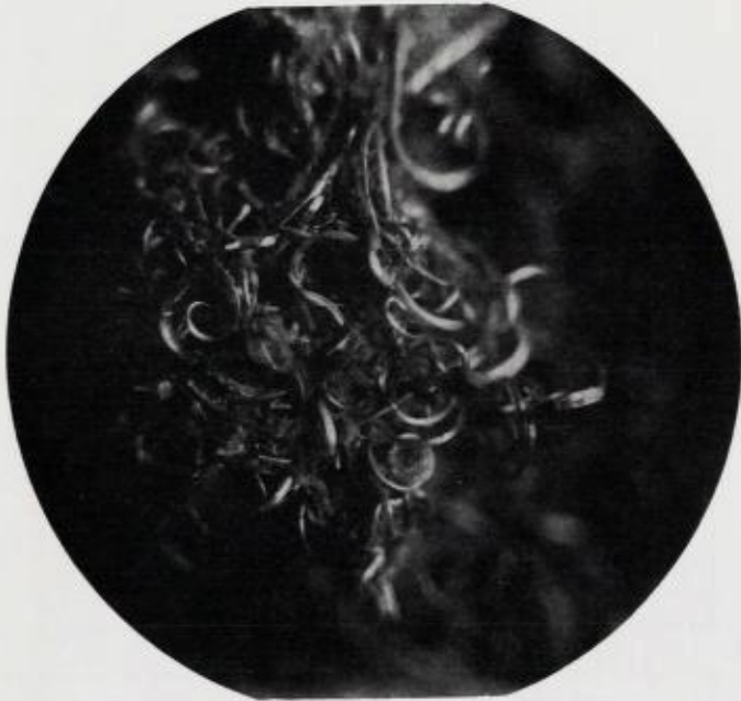
Fig. 5. Malachite in threads as pseudomorphs after native copper. From a sulphide-bearing quartz - breccia vein in Lassedalen.
