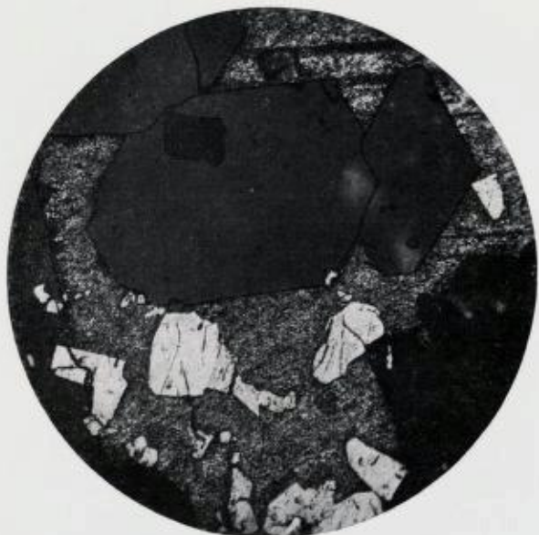
Phot. 1. Pyrite (white) showing euhedral crystals with reference to quartz (dark grey), and quartz with reference to native silver (strongly tarnished). 100 \times . Mine Bratteskjerpet, 112 m level.
