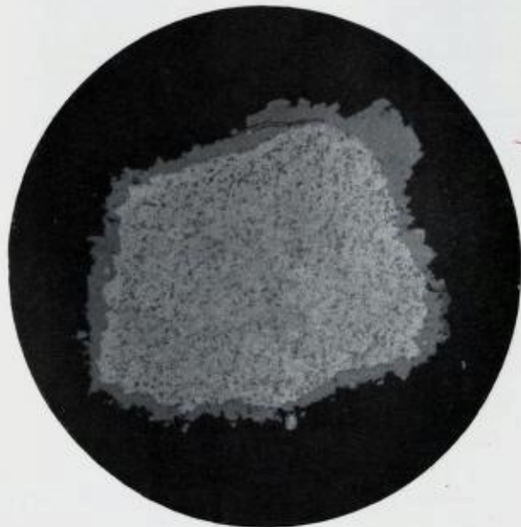
Phot. 16. Coating of rammelsbergite (grey) around a thread of native silver (white, tanished). Calcite (black). 300 \times . Mine Cristian VII. 150 m level.
