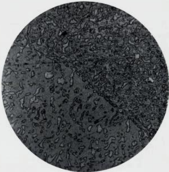
Phot. 12. Native silver (white) replaces marcassite which is partly rendered to pyrite (grey). Note border between twin crystals of marcassite. 200 \times . Mine Kongens grube. 520 m level.
