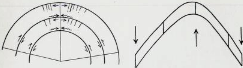
Fig. 15. (a) Diagram showing a bent fold. (b) Diagram of a shear fold. (After E. Cloos 1937.)
