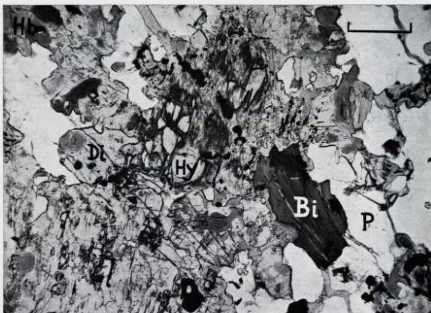
Fig. 2. Thin section of an arendalitic inclusion in the Herefoss granite. Ordinary light. The line measures 0,5 mm. P - plagioclase, Bi - biotite, Hy - hypersthene, Hb - hornblende, Di - diopside?. Arendalit inneslutning i granitten.
