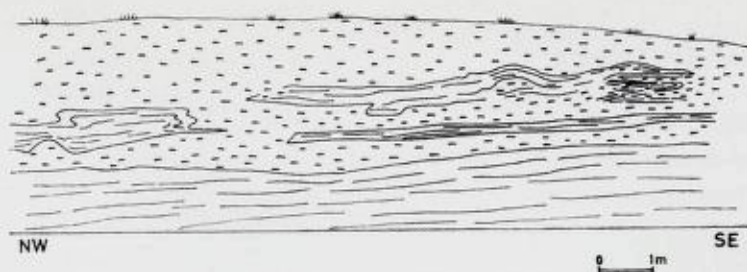
Fig. 5. Veined quartz-monzonitic gneiss interlayered with foliated quartz monzonite. The quartz monzonite is foliated parallel to the veined gneiss and permeates folds in the veined gneiss. Unless otherwise designated all symbols are the same as in Fig. 41.
