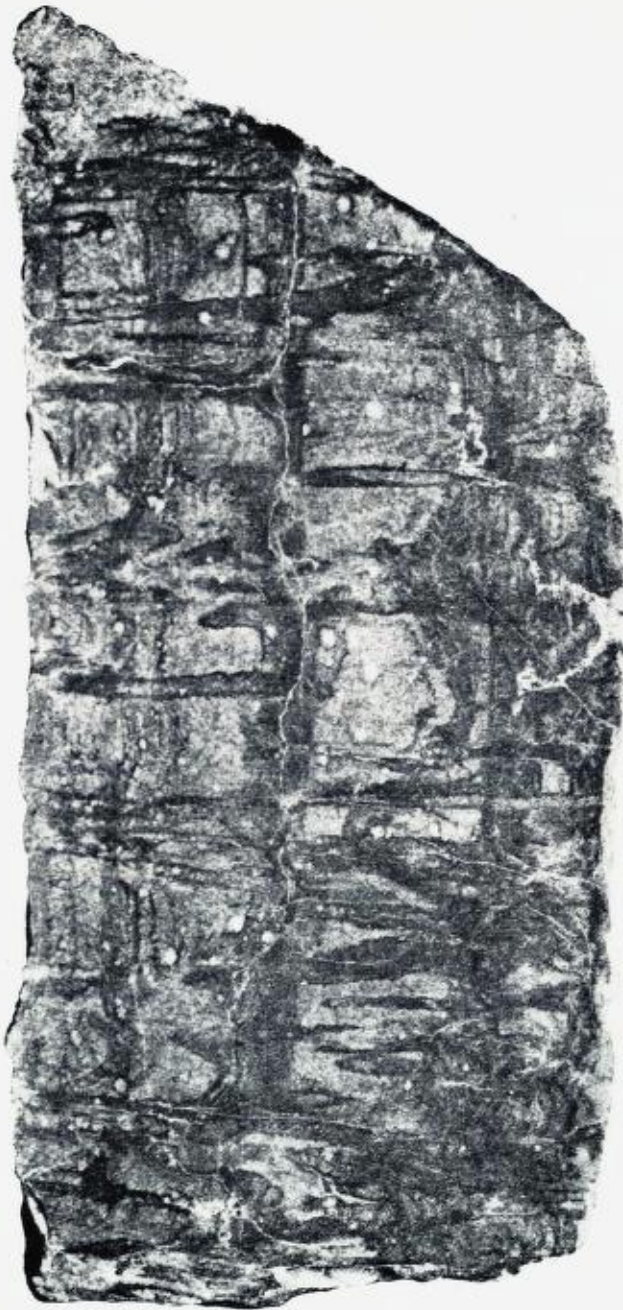
Fig. 9. Vertical section showing the "pipe rock" at Furnes Hospital. The light spot contain fluorite. \frac{2}{3} nat. size.
