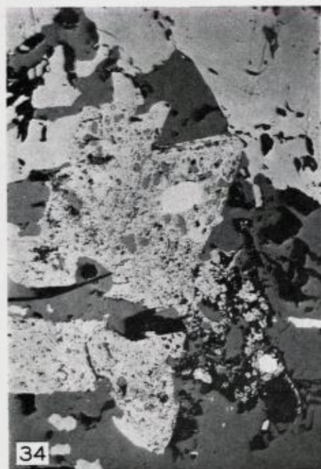
Figure 30. Part of semigraphic intergrowth between galena (medium grey, scratched) and «fahlerts» (dark grey) with fine-grained intergrowth of gudmundite (lightest) and pyrrhotite (slightly darker than galena). Reflected light, oil. 720x.
