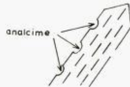
Fig. 4. Subangular analcime crystals idiomorphic against hornblende.
