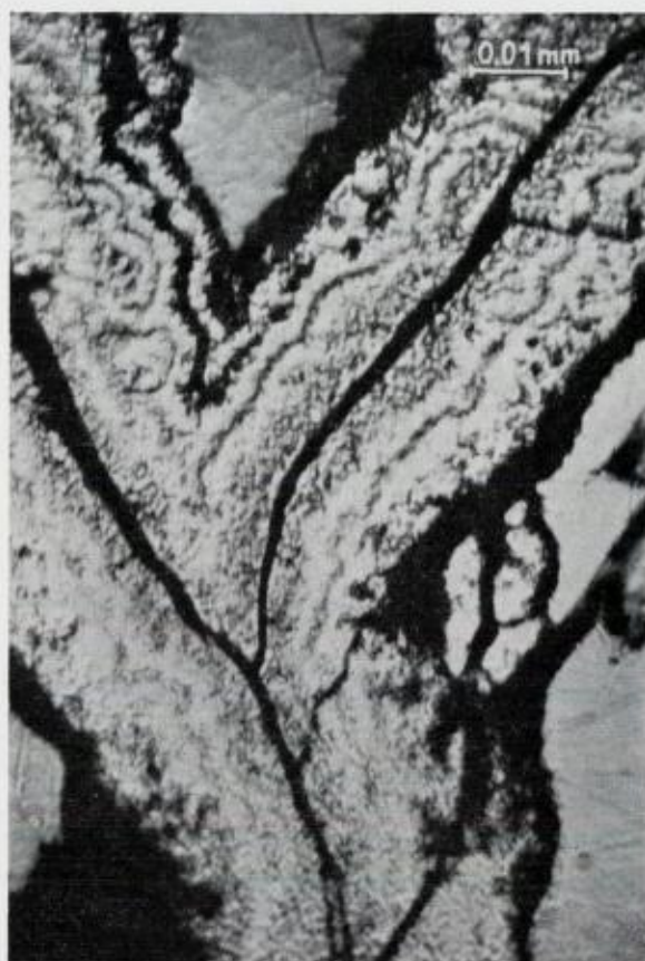
Fig. 15. Secondary pyrite along cracks in pyrrhotite.
