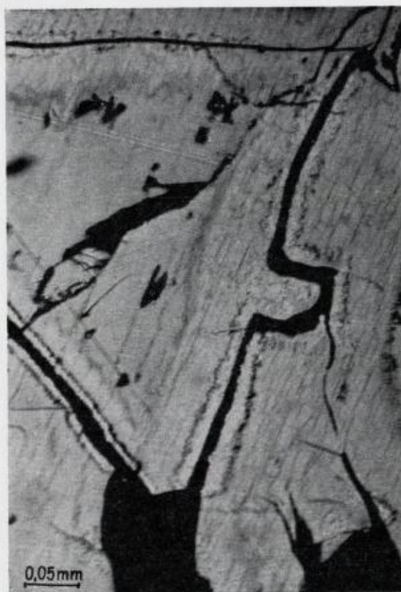
Fig. 14. Secondary pyrite (white) and marcasite (light grey) along limonite (black)-filled cracks in pyrrhotite (grey).
