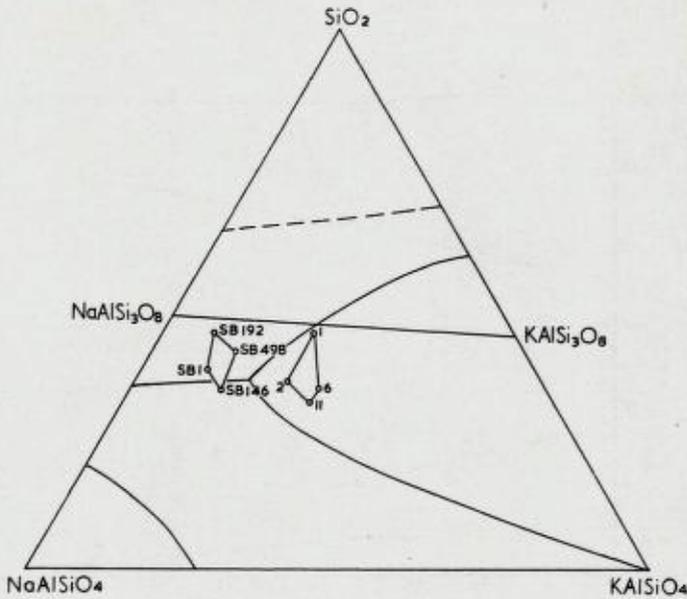
Fig. 60. Position of the analysed nepheline syenites in the system  $\text{NaAlSi}_3\text{O}_8$ — $\text{KAlSi}_3\text{O}_4$ — $\text{SiO}_2$ . Söröy analyses SB.1, SB.146, SB.192 and SB.498. Stjernöy analyses 1, 2, 6 and 11 (taken from Heier 1961).
