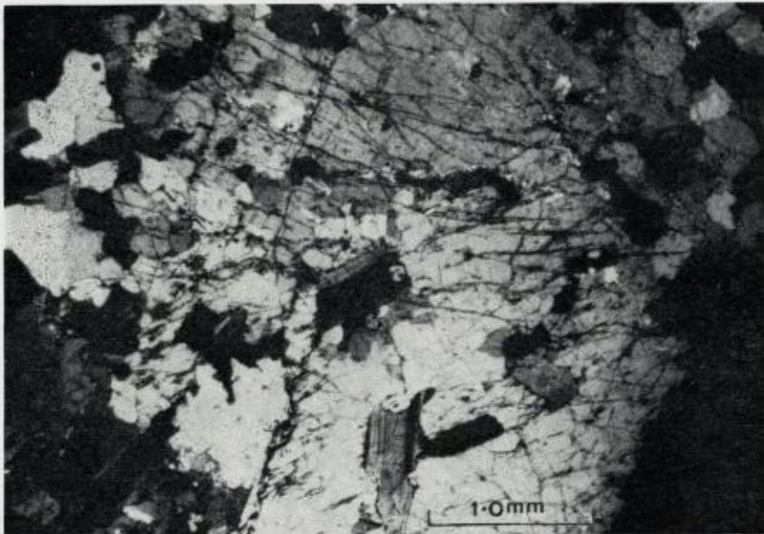
Fig. 9. Nepheline porphyroblast containing oriented inclusions of plagioclase. X-polarized light. (Slide no. SB.44.)
