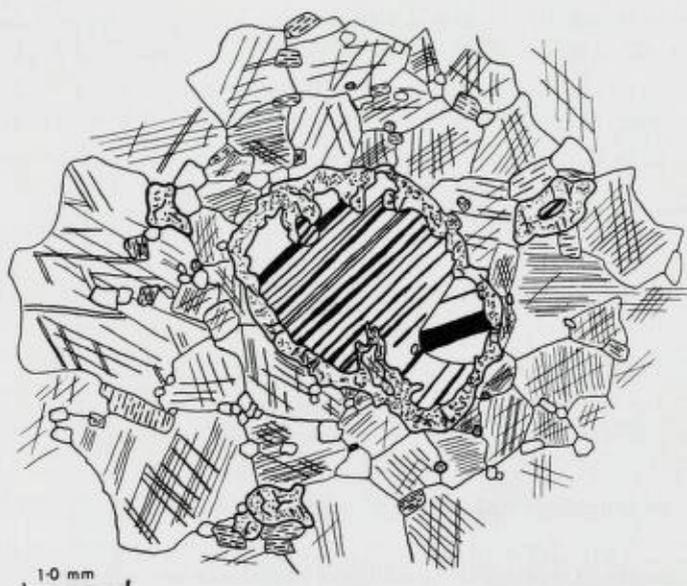
Fig. 59. Thin section of intrusive carbonate rock, showing andradite corona about plagioclase (bytownite). The ground mass is mainly calcite with some apatite and hedenbergite. Slide no. SB710.
