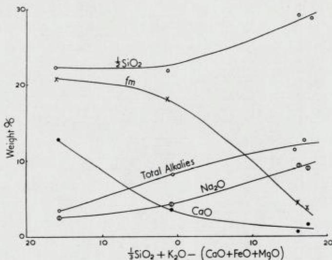
Fig. 63. Chemical trends of nephelization of metagabbro shear zones, shown by the plot of analyses of average gabbro (from Stumpfl and Sturt 1964), biotite schist, and two nepheline syenite gneisses. (Plotted on Larsen-type diagram.)
