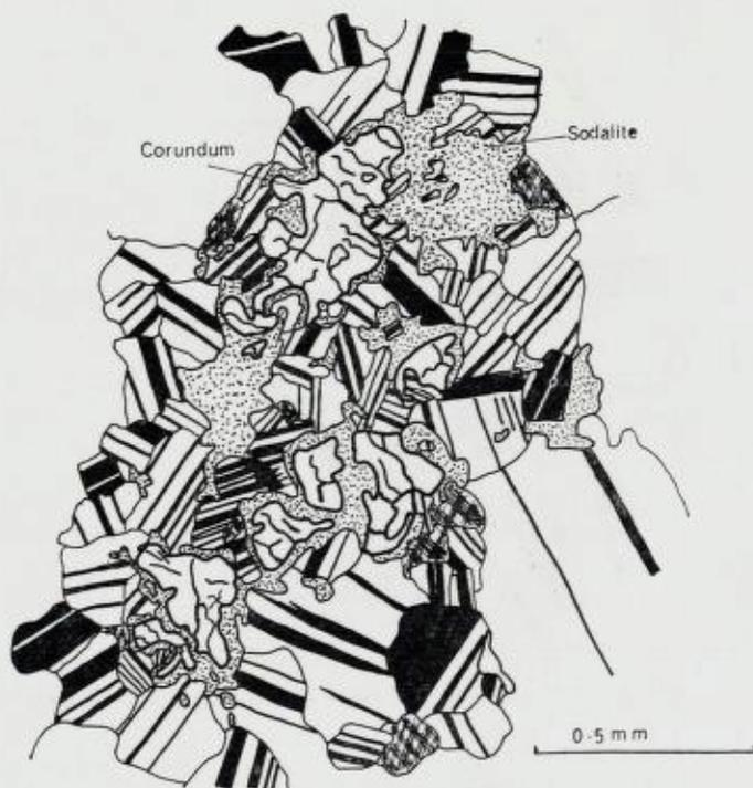
Fig. 32. Sodalite and corundum formed from albite/oligoclase. Nepheline syenite gneiss. (Slide no. SB.481.)
