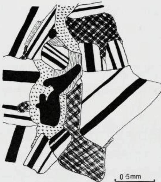
Fig. 33. Sodalite (crosses) and late biotite formed about pyrite. Nepheline syenite gneiss. (Slide no. SB481.)
