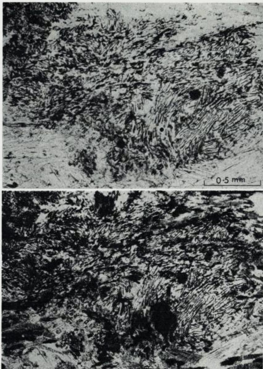
*Fig. 13. Muscovite containing oriented corundum rods, the orientation being independent of that of the muscovite. (Slide no. SB.535.)*
