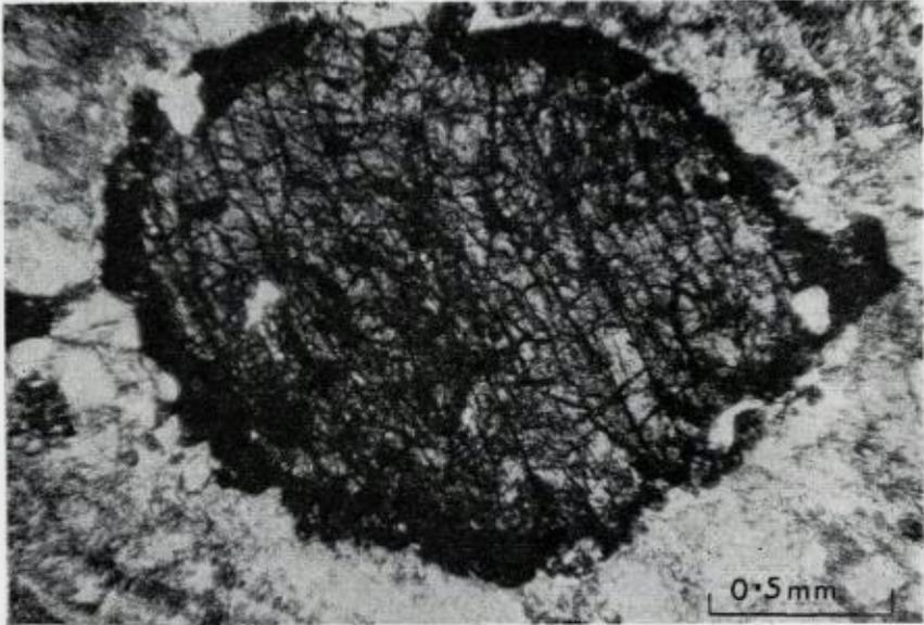
*Fig. 39. Aegirine-augite crystal rimmed by ferro-bastingsite in shonkinite. Plane polarized light. (Slide no. SB.91.)*
