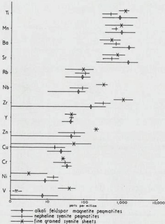
Fig. 64. Trace element distribution in intrusive phases of the Nepheline Syenite Association. The range and average values are given in parts per million.
