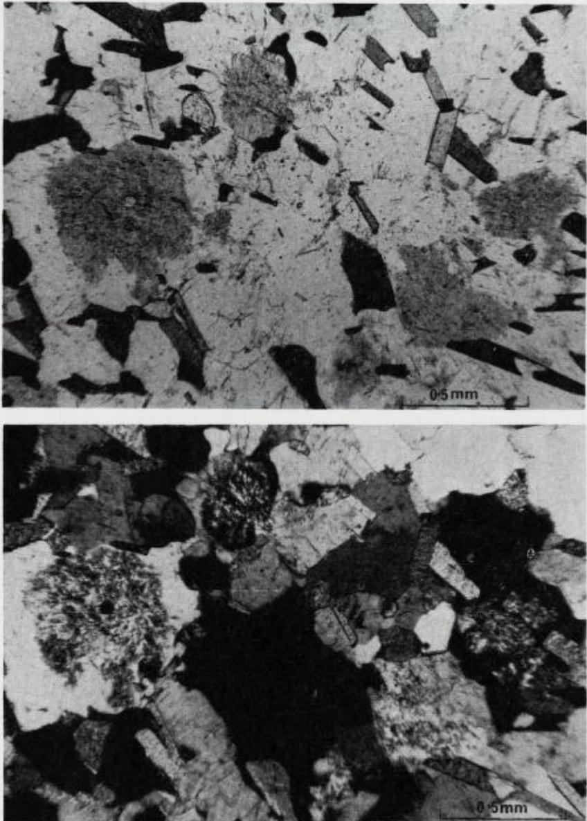
*Fig. 3. Photomicrographs to show corroded basic cores to albite-oligoclase in alkali-gneiss (albite/oligoclase, microcline, biotite, apatite). (Slide No. SB102.)*
