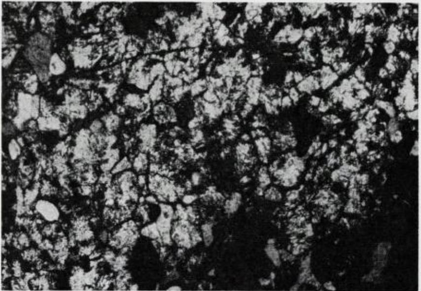
*Fig. 45. Relict grain boundary pattern (feldspar) preserved in completely zeolitized sbonkinite. (Slide no. SB.64.)*
