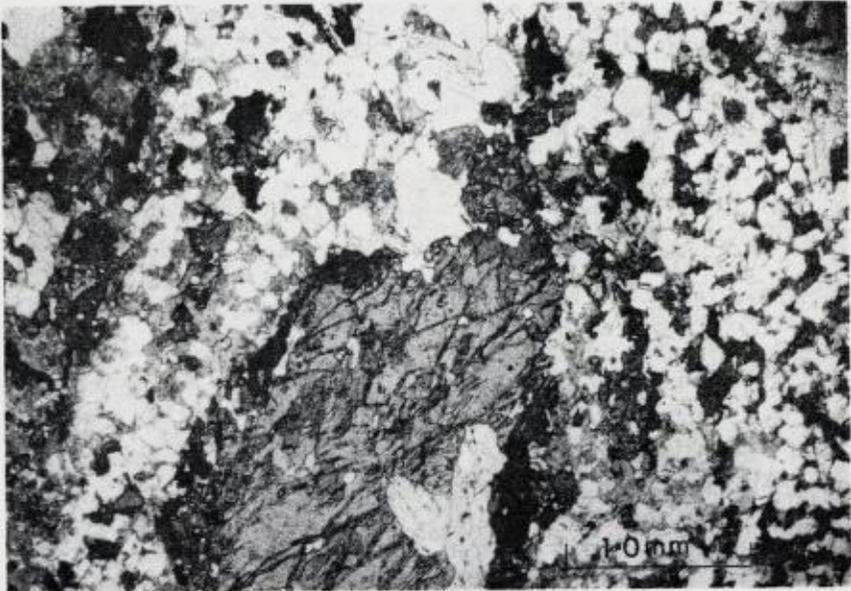
*Fig. 40. Aegirine-augite crystal rimmed by bastingsite, but also containing inclusions of bastingsite of different orientation. Note the partial zeolitization of the groundmass feldspar mosaic. Shonkinite. Plane polarized light. (Slide no. SB.5.)*
