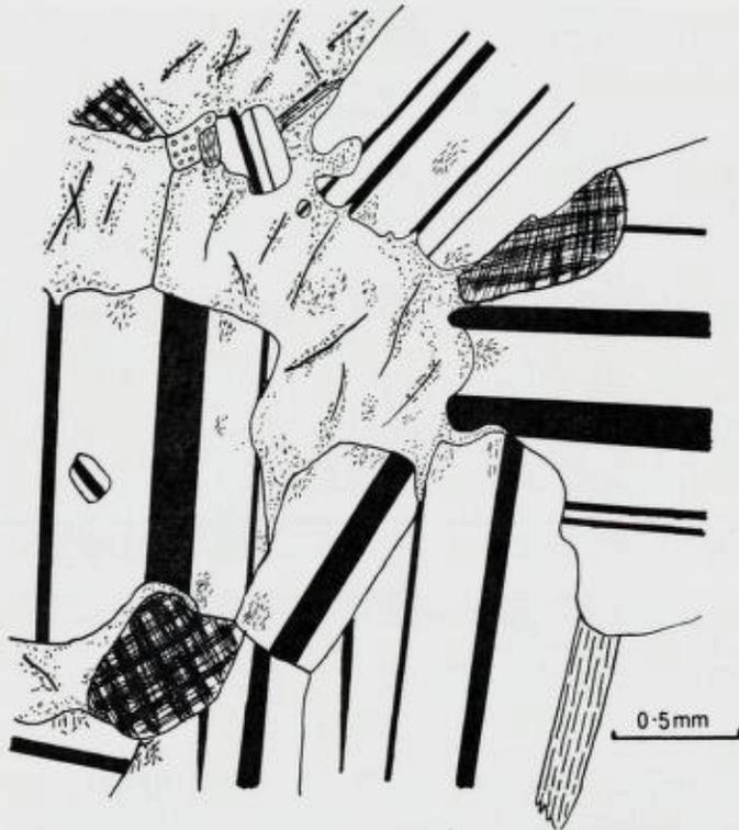
Fig. 8. Thin-section of nepheline syenite gneiss illustrating late growth of nepheline (stippled). Nepheline is seen to form along grain boundaries, and to preferentially replace certain plagioclase twin lamellae (Slide no. SB.51).
