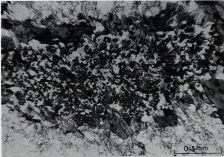
Fig. 14. Patch of albite and corundum surrounded by biotite in fenitized semi-pelite. Plane-polarized light. (Slide no. SB.536.)
