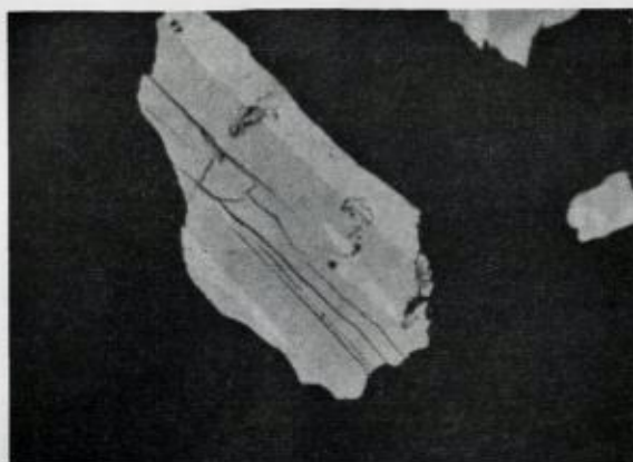
Fig. 9. Pyrrhotite (medium grey) with lamellae of pentlandite (white). Chalcopyrite (light grey), gangue (black). Breivikbotn. Magnif. 330 \times , Oil immersion.
