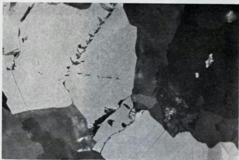
Fig. 7. Rutile (light grey) and sphene (dark grey rim) after ilmenite. Breivikbotn. Magnif. 330 \times . Oil immersion.
