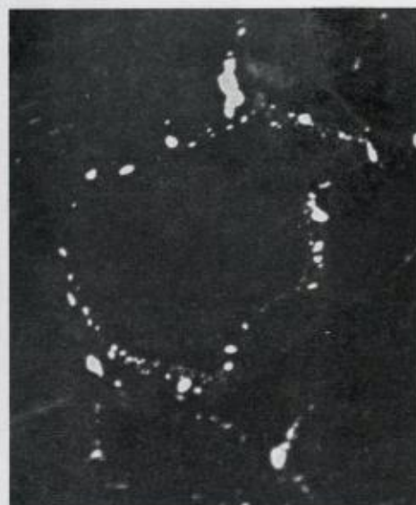
Fig. 11. Ilmenite with corona of sphene (reflection pleochroism). Storelv. Magnif. 90 \times .
