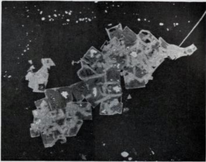
Fig. 10. Pyrite cubes (white), nearly completely altered into goethite ( \alpha -FeOOH; dark grey) and lepidocrocite ( \gamma -FeOOH; light grey). Breivikbotn. Magnif. 230 \times , oil immersion.
