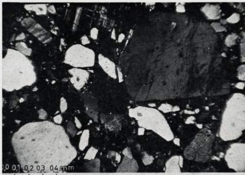
Fig. 16. Thin section photomicrograph of Moelv tillite. Note angular grains.
