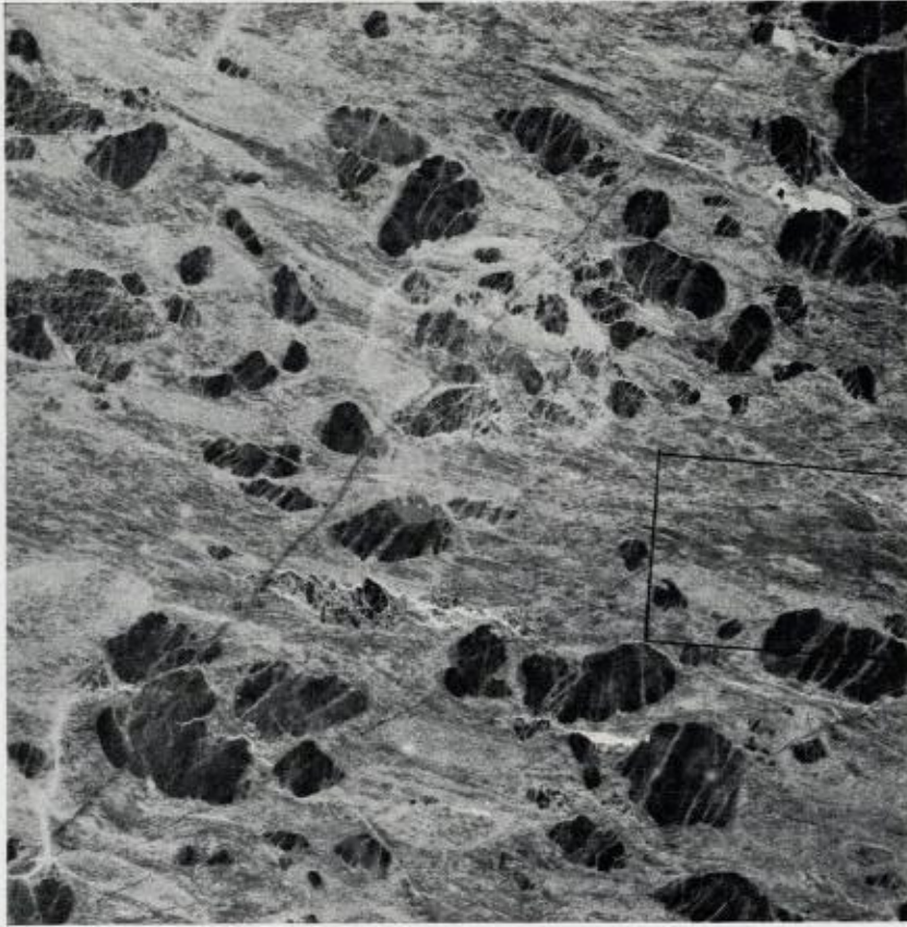
Fig. 3. Tension joints in quartz grains with calcite matrix. (Framed figure 4 a.)
