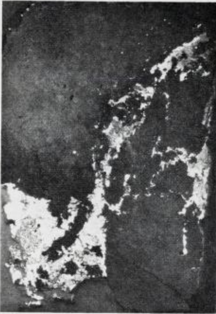
Fig. No. 13. Magn. ca. 3X. Lead-rich quartz deposition in wall rock. Lateral secretion directly connected with brecciated zinc-rich ore. White — galena. Light grey, strongly cracked — sphalerite. Dark — mainly quartz.
