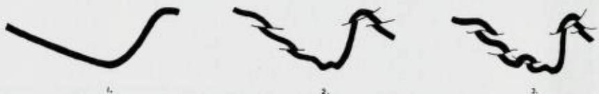
Fig. 5. Illustration of the suggested progressive development of the late f_2 thrust faults as a response to the tightening of the f_2 buckle folds.
