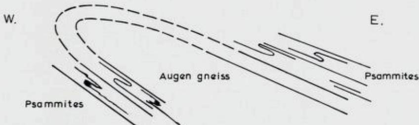
Fig. 1. Section of the  $F_1$  anticline on the south of Skjervøy. The sense of vergence of the minor folds indicates that the anticline closes and faces west. The axis plunges gently to the south-east.
