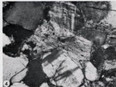
Plate 3 Fig. 3. Rounded feldspar grain projecting into adjacent quartz grains. Feldspathic sandstone of the "Hyolithes Zone". Crossed polarisers. X94.
