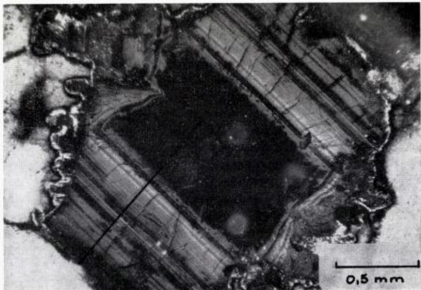
Fig. 5. Polished section of complex titanium mineral in polarized light, oil immersion.
