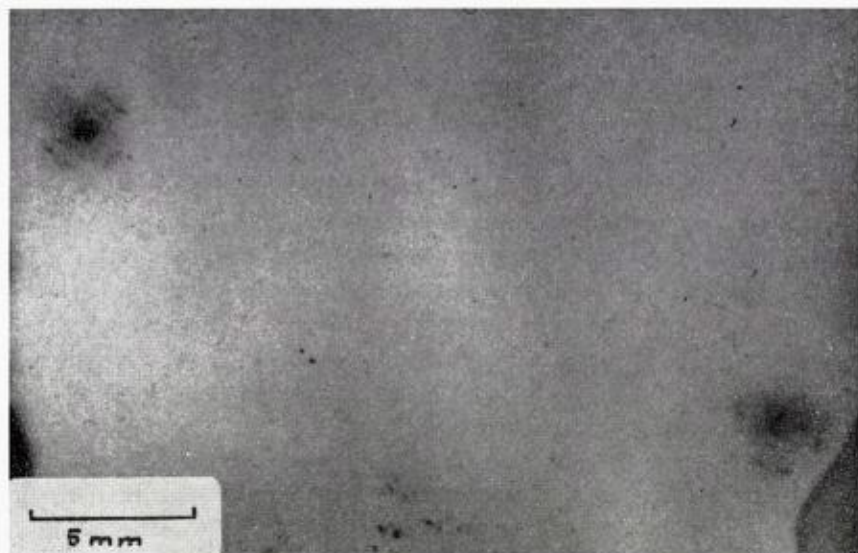
Fig. 9. Auto-radio exposure of polished fels containing two grains of complex titanium mineral.
