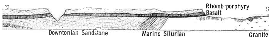
Fig. 1. Section along the Lier valley to the east side of Tyrifjord. Permian sediments below the lavas are not marked. A Permian sill of quartz porphyry (marked in black) is locally found below the lavas (after Kjerulf 1879, Holtedahl et al. 1934).
