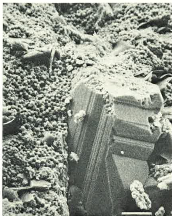
Fig. 14. SEM-picture of re-textured pyrite ('Rogenpyrit') formed by coalescence of frambooids, in stage of porphyroblastesis. From pyritic 'vasskis'-ore, Kalddalen prospect VII, Rennebu. Scale bar: 5 \mu m.
