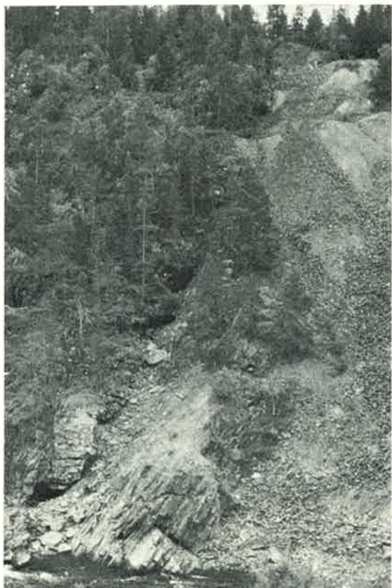
Fig. 15. Nyberget mine, Innset. View to the south. Note the inclined trench with rock pillars in the pyrite ore, and footwall amphibolite exposed in the lower part of the hillside.
