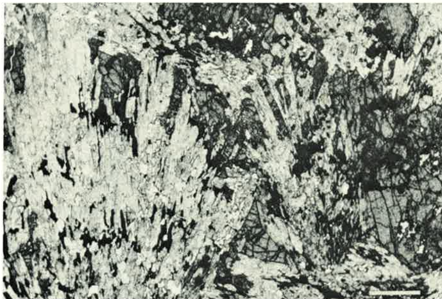
Fig. 7. Pyrrhotite disseminations within magnetite-grunerite iron-formation at Gråhø (85). Note bundles of grunerite intersecting garnet porphyroblasts. Plane polarized light. Scale bar: 1 mm.
