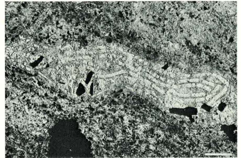
Fig. 19. Contorted, glassy microband of a probable colloidal origin. From the 'black fels' at Hakefjellet prospect, Rennebu. Magnetite (black) in a dark chloritic matrix. Plane polarized light. Scale bar: 100 \mu m.
