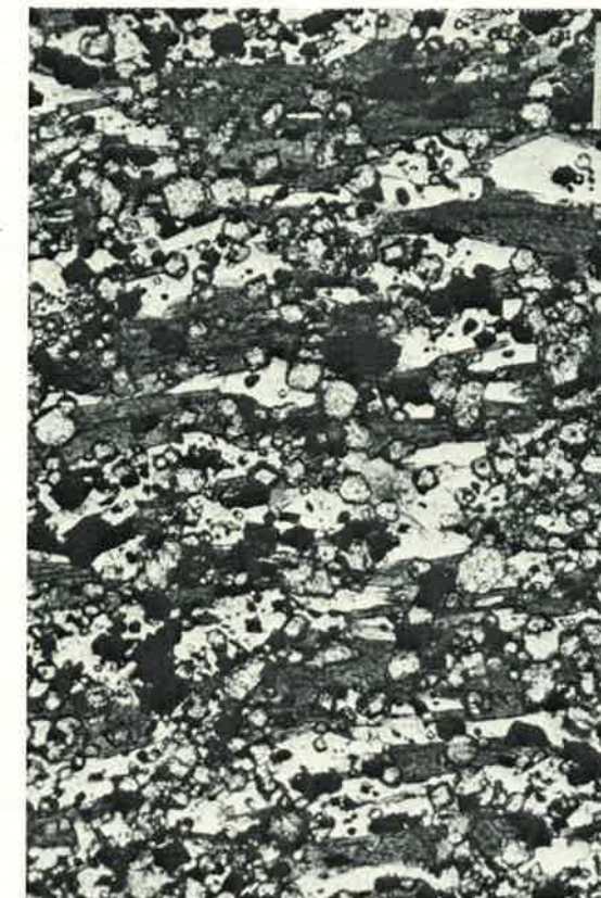
Fig. 6. Garnet-magnetite-biotite schist from the iron-formation at Lomnesvola (113). Plane polarized light. Scale bar: 100 \mu m.
