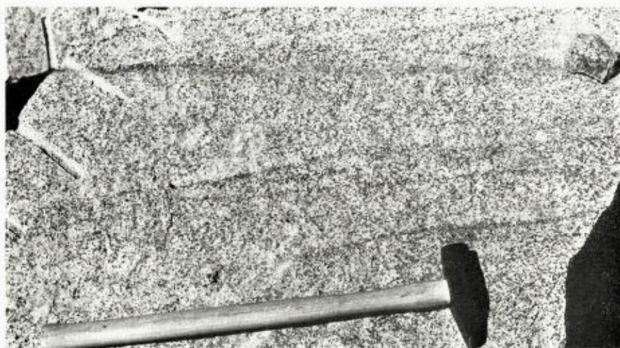
Fig. 4. Block of trondhjemite from the main quarry at Follstad showing biotite streaking and faint foliation. The trondhjemite is usually very homogeneous and massive.
