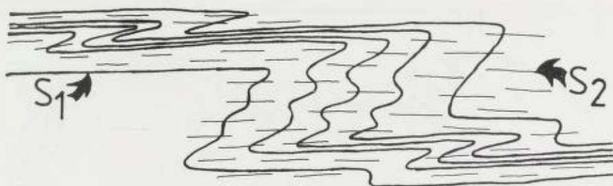
Fig. 4. Schematic figure showing typical style of asymmetric D_2 fold with strongly flattened long-limbs and open buckle-folds in the steep middle-limb.
