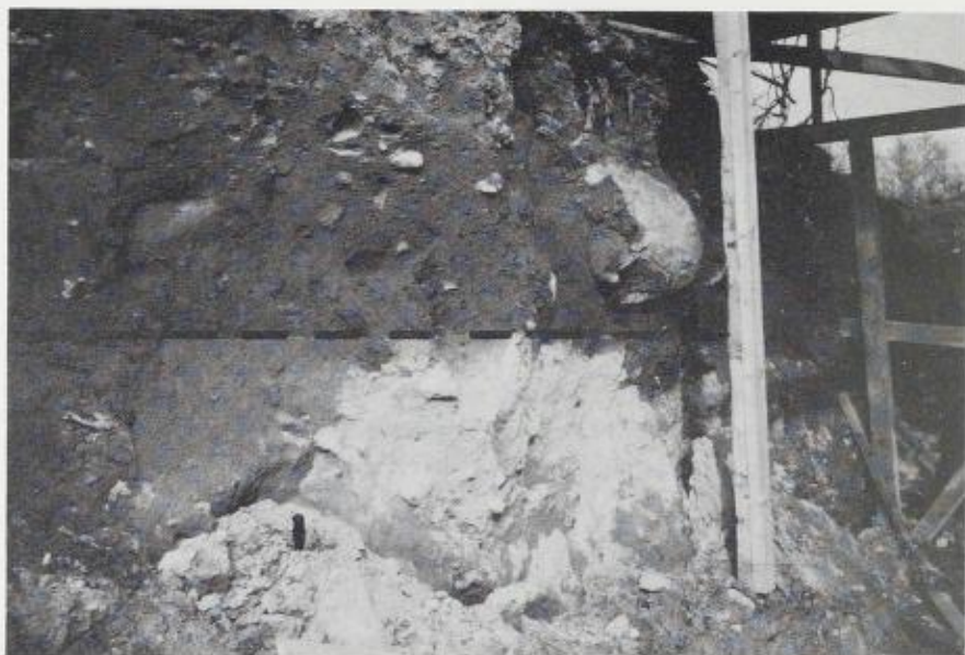
Fig. 3: Kautokeino slakteri. Grensen mellom undre (20 ø ) og øvre (380 ø ) morene er stiptet. Mellom morenene ligger en 2–8 cm tykk brunfarget diamikton, Kautokeino butchery. The boundary between lower (20 ø ) and upper (380 ø ) till is marked with a broken line. A 2–8 cm thick brownish diamicton separates the two tills.
